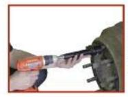
Allows you to clean the full length of the thread on 10 wheel studs in 3 minutes or less.
